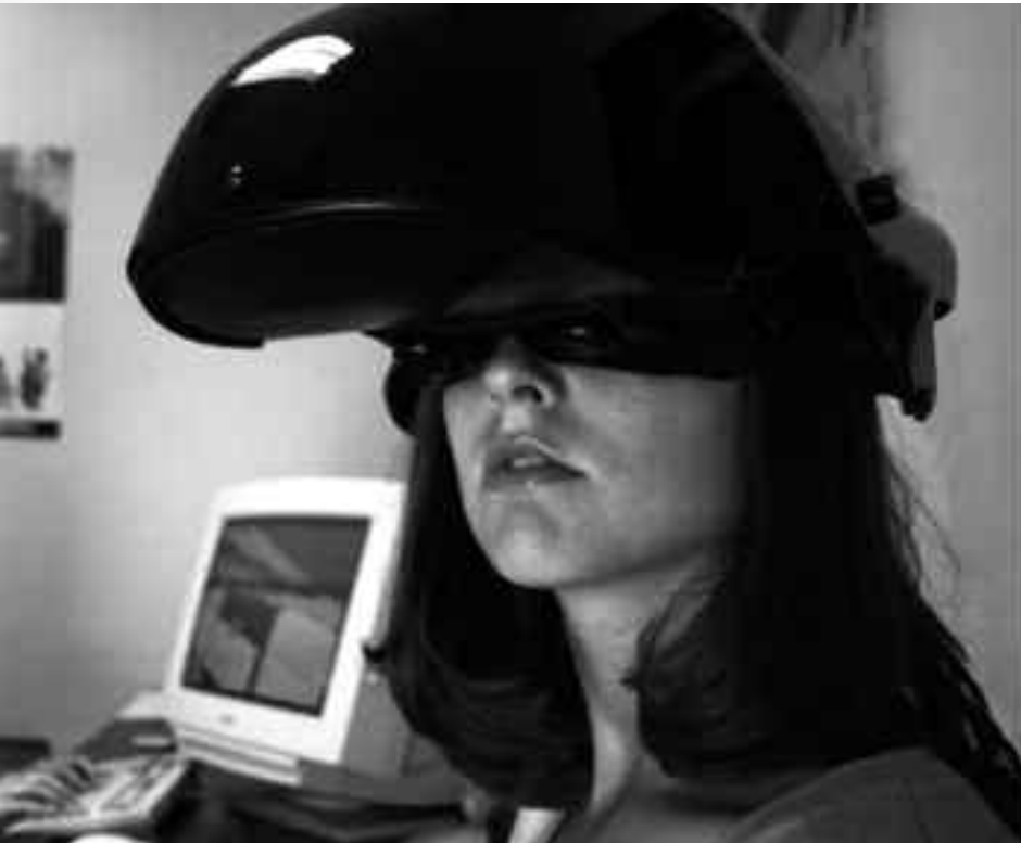
▲ The Client wears a headmounted display with small monitors to receive both visual and auditory cues
